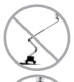
Do not raise or extend the boom unless the machine is on a firm, level surface.
