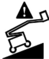
If the tilt alarm sounds when the platform is raised, the Machine Not Level LCD symbol will come on and the drive function in one or both directions will not operate. Identify the condition of the boom on the slope as shown below. Follow the steps to lower the boom before moving to a firm, level surface. Do not rotate the boom while lowering.
