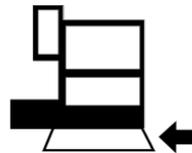
If the platform bumper comes into contact with an object, the machine will shut down and no functions will operate.
