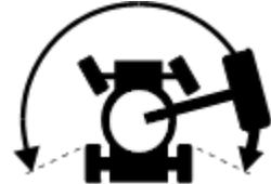
Note: When the drive enable system is in use, the machine may drive in the opposite direction that the drive and steer control handle is moved.
