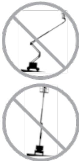
Do not raise or extend the boom unless the machine is on a firm, level surface.
