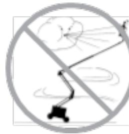
Do not raise the boom when wind speeds may exceed 28 mph/12.5 m/s. If wind speeds exceed 28 mph/12.5 m/s when the boom is raised, lower the boom and do not continue to operate the machine.
