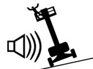
To restore drive functions, follow the boom lowering process, explained in the previous procedure.
