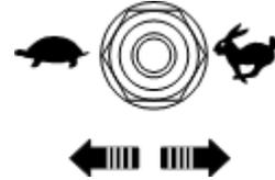
Note: Function speeds will increase or decrease by 5% each time the function speed control switch is moved. The speed control switch can also be held in either direction to increase or decrease function speed.
