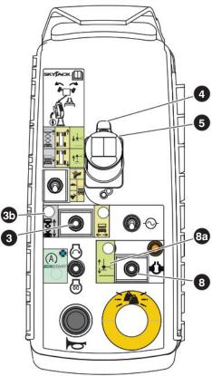
11. Move the lift/off/drive switch 3 to the lift position 3.
