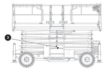
Figure 10 Approximate center of gravity
