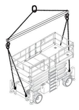
Figure 09 Appropriate method to hoist
