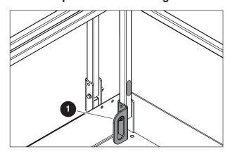
1 Fall-protection anchorage: When required, use this as a point to attach personal fall protection equipment (PFPE). Do not attach the PFPE to any other points on the platform. Do not use this anchorage to lift, anchor, attach, or hold the platform, or other apparatuses or material.
