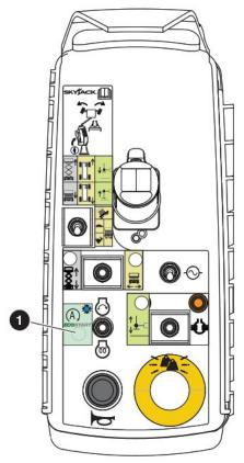
Figure 04 ECOStart light on the platform control console
