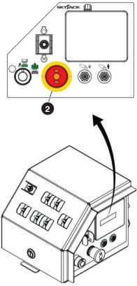
4.3-6 Do a test of the emergency-lowering function
