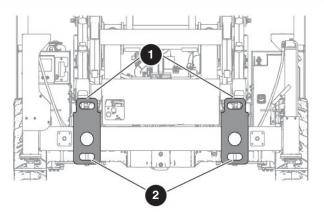
Figure 08 Lift and tie-down points
