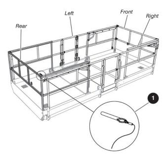
1 Guardrail lock-pin with lanyard: Use this pin to lock the guardrails.
