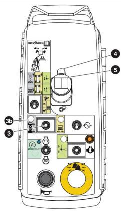
4.3-19 Do a test of the SGLE switch (optional equipment)
