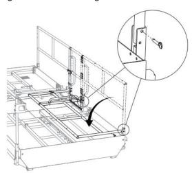
**16.** Pull the gate latch, and fold down the front-left guardrail along with the left gate.
