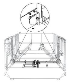
**15.** Remove all the **lock-pins** on the front-left guardrail and the left gate.
