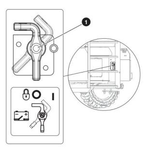
Main power disconnect: This switch disconnects power to all control circuits when it is in the off position. The switch must be in the on position to operate the MEWP. The switch must be in the off position when you transport the MEWP or put it in storage. Section 3 – Familiarization Control functions
