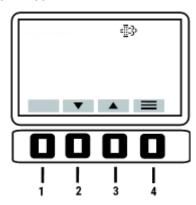
5 Using the control buttons 2 and 3 below the LCD screen, select "Diagnostics" from the Main Menu. Press the control button 4 to confirm the selection.
