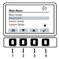
6 Using the control buttons 2 and 3 below the LCD screen, select "Regen Menu". Press the control button 4 to confirm the selection.
