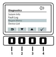
7 Using the control buttons 2 and 3 below the LCD screen, select "Initiate Regen". Press the control button 4 to confirm the selection.
