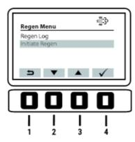
8 The LCD screen will display the message "Initiate Regen". Press the control button 4 to confirm.
