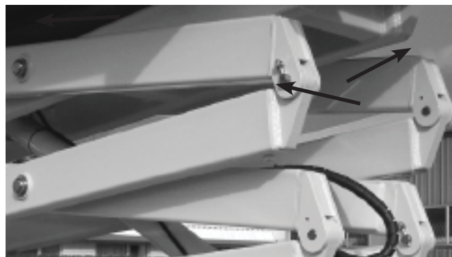
Figure 7.19 - Structural Damage and Welds
