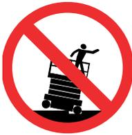
Do NOT Operate a Stowed MEWP Within 4ft (1.2m) of Any Drop-off or Hole
