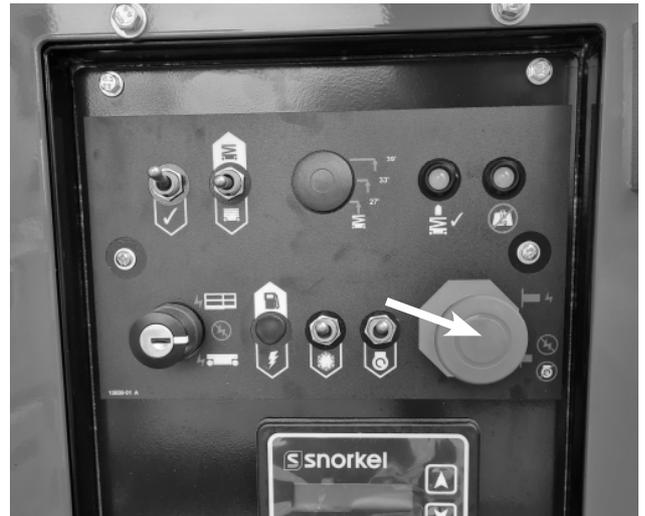
**Figure 4.2 – Lower Controls Emergency Stop Switch**
