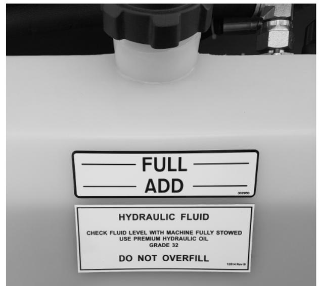
Figure 5.3 Hydraulic Oil Tank
