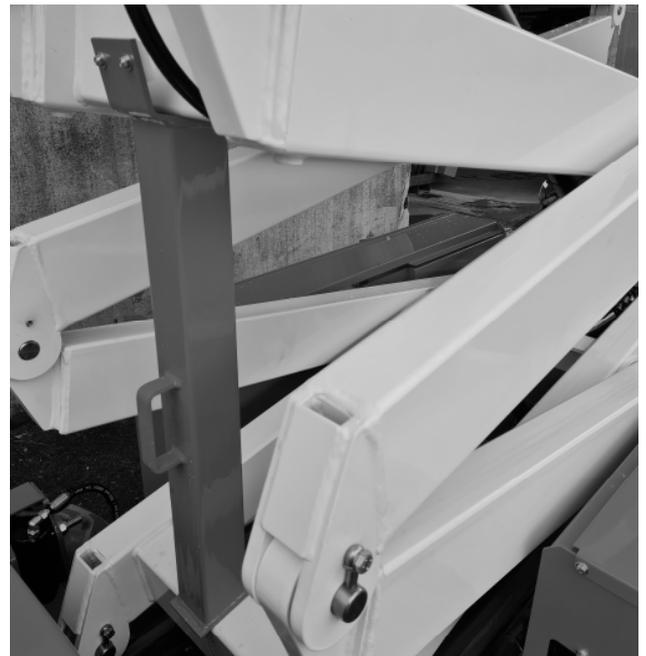
**Figure 7.2 – Safety Prop in Support Position**
