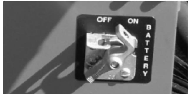
Figure 10.2 – Battery Disconnect Switch
