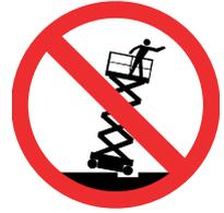
Do NOT Operate an Elevated MEWP Within 4ft (1.2m) of Any Drop-off or Hole
