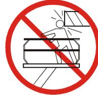
**NEVER** position the platform without first checking for overhead obstructions or other hazards.
