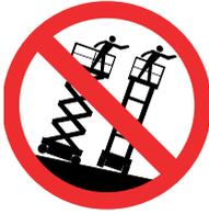
Do NOT Drive an Elevated MEWP on Soft, Uneven or Sloping Surfaces
