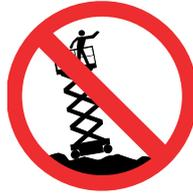
Do NOT Operate an Elevated MEWP on Rough or Uneven Terrain
