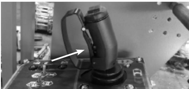
Figure 4.8 – Joystick Interlock Switch
