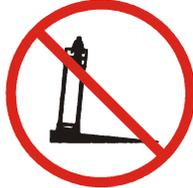
**NEVER** elevate the platform or drive the machine while elevated unless the machine is on a firm, level surface.
