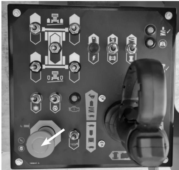
**Figure 4.1 – Upper Controls Emergency Stop Switch**
