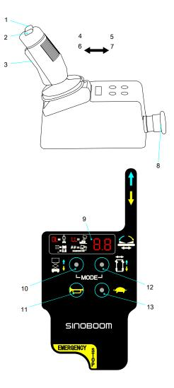
Figure 6-3 Platform controller (DTC)
