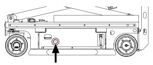
Figure 7-1 Power off switch
