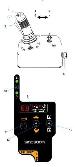
Figure 6-2 Platform controller (SINOBOOM)
