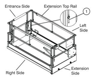
Figure 3-11a. Folding Guardrail System
