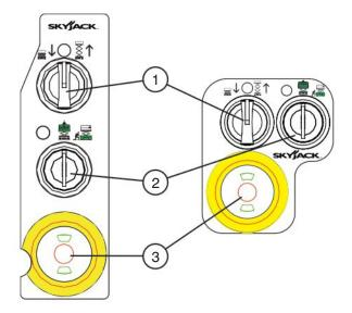
Figure 2-2. Base Control Console
