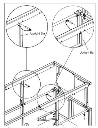
Figure 3-10. Variable Position Manual Extension Platform
