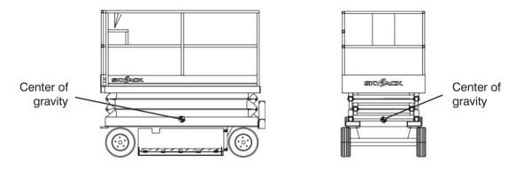
Figure 3-13. Center of Gravity
