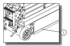
Figure 3-3. Pothole Protection Device
