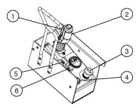
Figure 2-6. Platform Control Console
