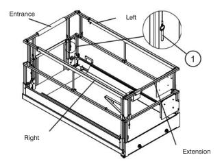
Figure 3-5. Folding Guardrail System
