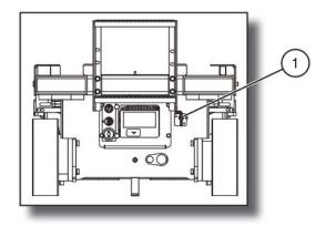
Figure 2-1. Main Power Disconnect Switch
