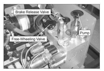
Figure 10.3 - S1930E/S1932E Hydraulic Tray
