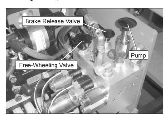
Figure 11.2 - S1930E/S1932E Hydraulic Tray
