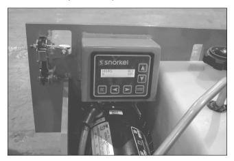
Figure 5.5 - Diagnostic Center LCD Display
