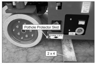
Figure 8.12 - Pothole Protector Skid
