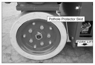
Figure 8.11 - Pothole Protector Skid
