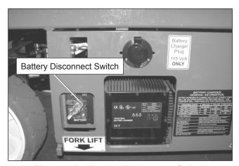
Figure 7.1 - Battery Disconnect Switch
