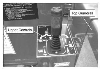
Figure 7.4 – Upper Control Operating Position
