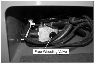
Figure 10.5 - S2632E Rear of Chassis
