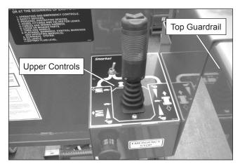
Figure 9.2 - Upper Control Operating Position
